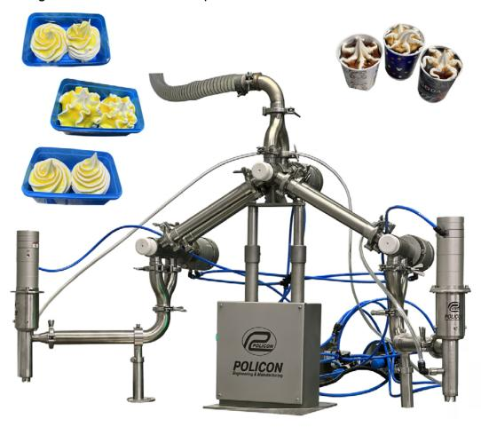
Dose adjustment is carried out for each position separately by measuring the dosing time. Ice cream supply to the dispenser is carried out from a continuous freezer
